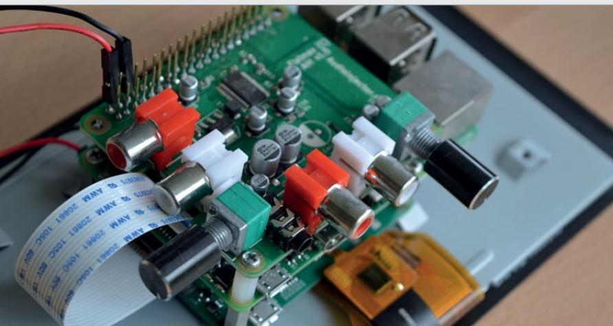
The Audio Injector stereo sound card adds line-level audio inputs to the Pi
