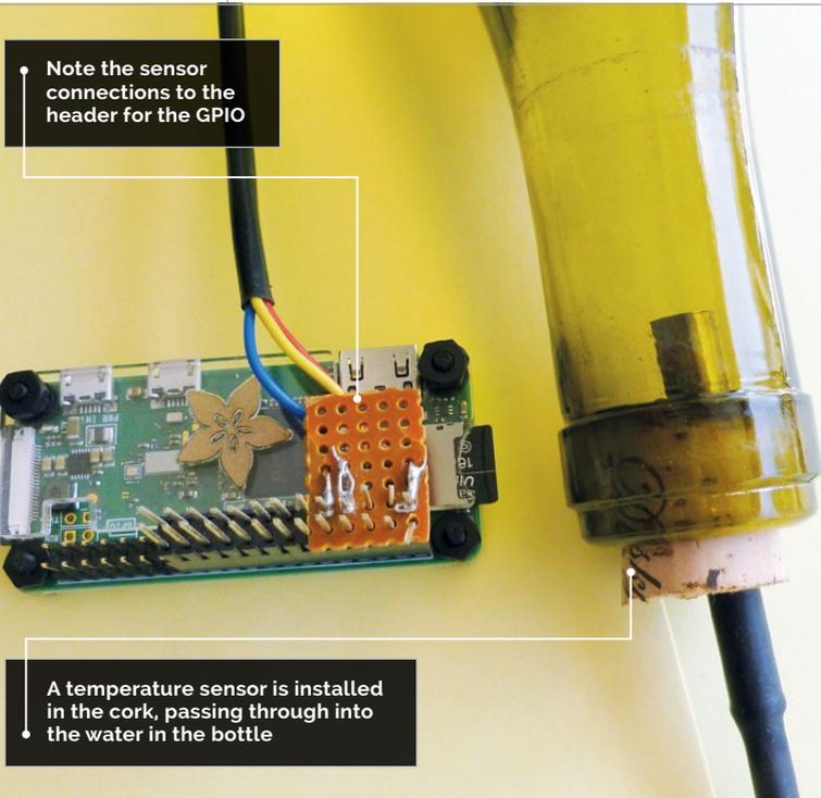
Note the sensor connections to the header for the GPIO
