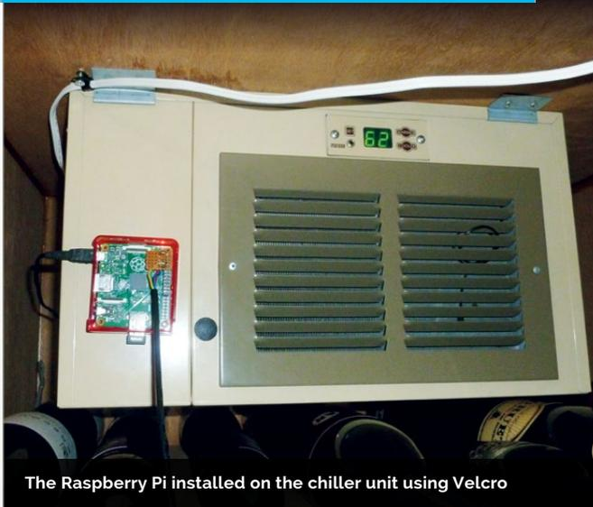
The Raspberry Pi installed on the chiller unit using Velcro
