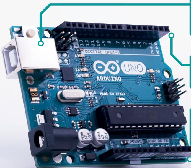
Power the Arduino from one of the Pi's USB ports; this also enables two-way communication
