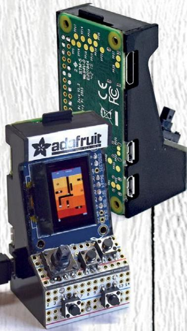
the oldest of arcade games. The buttons are soldered to some custom-made prototype boards, and the case is a custom design in laser-cut acrylic. Adafruit themselves say the design process was more of a challenge than anything else but hey, it would be a cool project to break out at a party.
