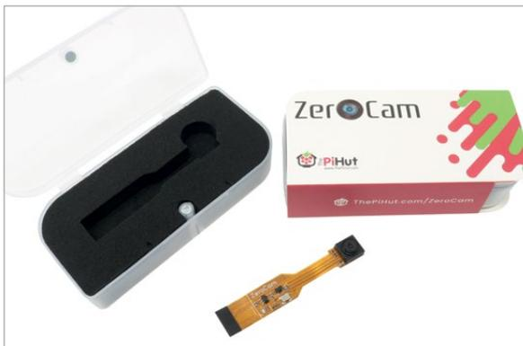
**Right** The ZeroCam is designed to fit the reduced-size camera connector on the Pi Zero
