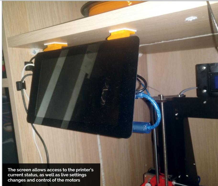
commands. One of the best features of the software is the fact that you can access the printer remotely via the local network by navigating to the Pi's IP address on any device connected to the same LAN. This allows you to upload files to the server to be printed, as well as allowing you to view the progress of prints and cancel them. You can also view a live picture feed of the printer if you connect a USB webcam to the Pi.
